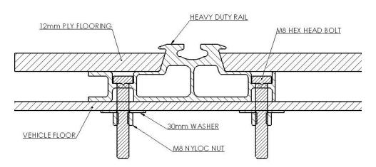
Available in 3.95 and 4.50 metre lengths, this rail profile can be installed with a maximum unsupported span of 600 mm under normal conditions.
